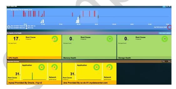
As we dig in, we can see the high CPU ready to be the root cause. The CPU ready time is about 44%.
