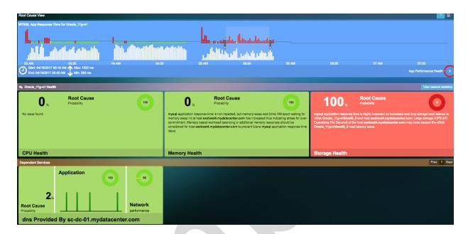
Digging in further, we discover the read latency to be very high. The IOPS is also being shared between multiple VM's on the same host. This can cause high latency on a single service.
